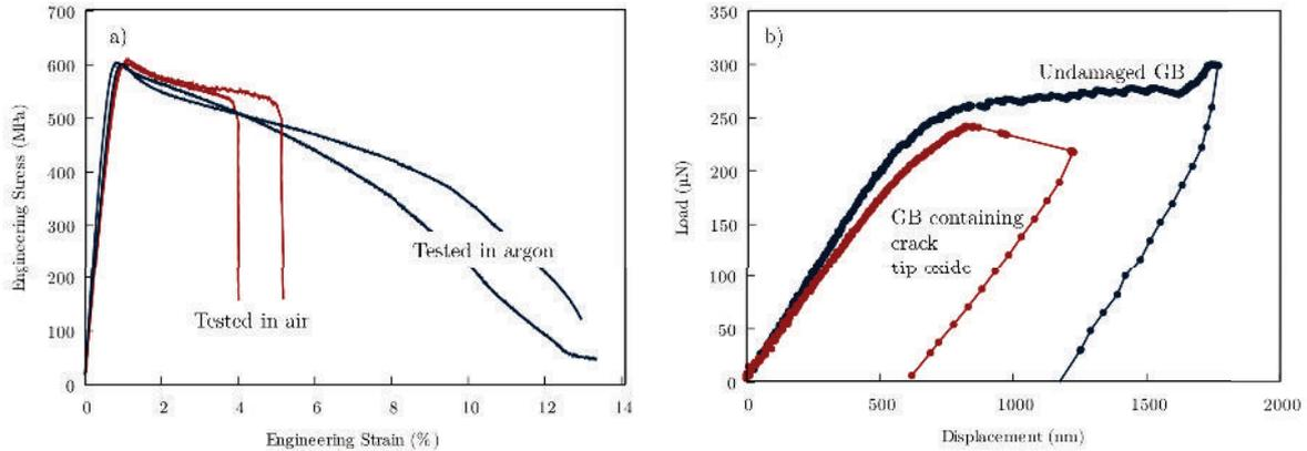
Figure 1: a): Slow strain-rate tensile stress-strain curves for alloy 720Li tested in oxygen and argon atmosphere. b): Load-displacement curves for a micro-cantilever containing a crack tip oxide and a reference micro-cantilever from bulk alloy 720Li.
