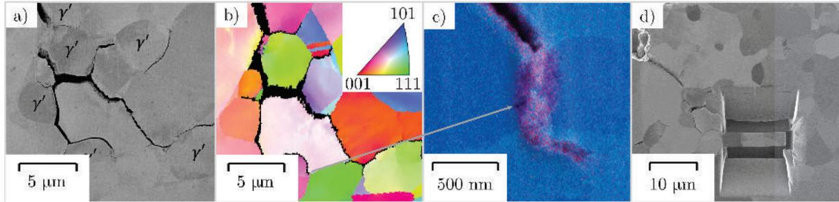
Figure 2: a): SEM image showing a crack connected with the fracture surface. b): EBSD image of the crack path. c): High resolution EDX of a isolated crack tip. Ni, Cr, Co, W and Mo are highlighted in light blue. Ti and Al are highlighted in dark blue and O is highlighted in red. d): FIB-SE image showing an untested micro-cantilever containing a crack tip oxide.
